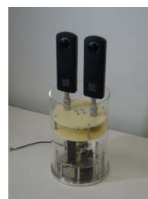
Figure 2: TwinCam head (fixed-azimuth rotation mechanism).
